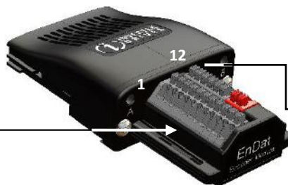
OPT-2-ENDAT2-IN Endat Absolute Encoder Connections OPT-2-SINCOS2-IN SinCos Encoder Connections
