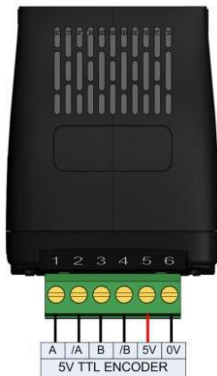
OPT-2-ENCOD-IN Connection Example – 5V TTL Encoder
