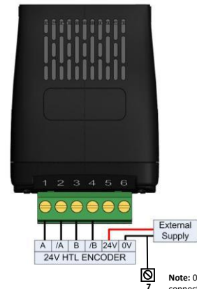
OPT-2-ENCHT-IN Connection Example – 24V HTL Encoder
